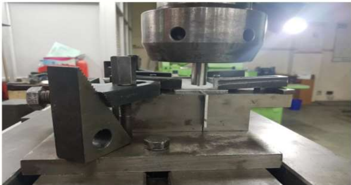
Figure Friction Stir Welding Fixture for Tailor blank fabrication.
